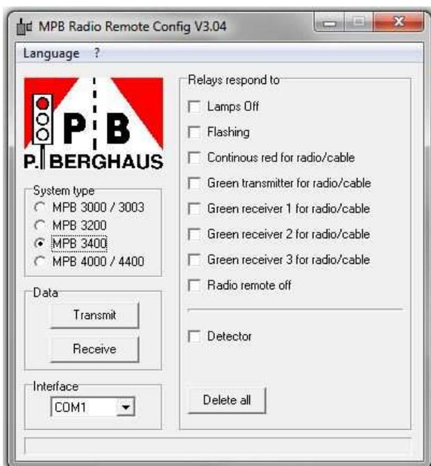
If the "**Detector**" box is ticked, the relay responds when the detector input is in use.
