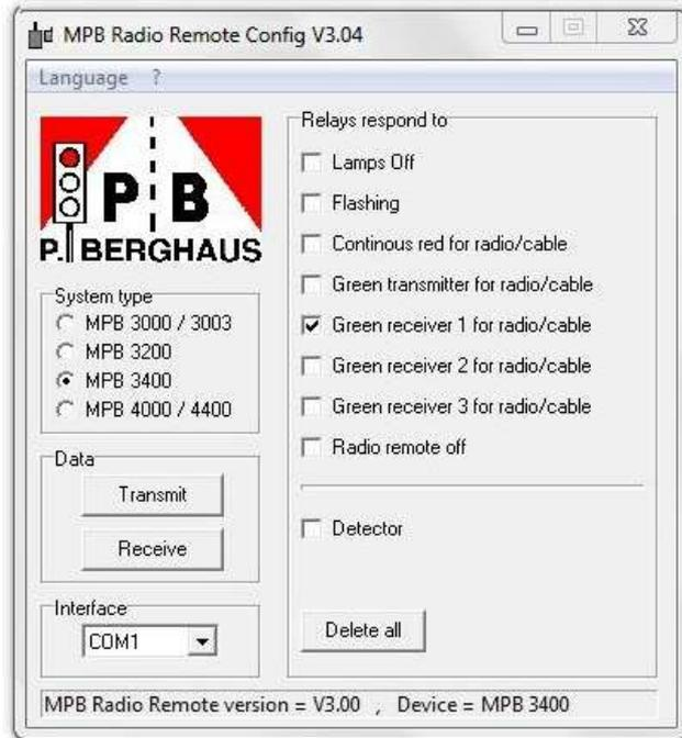
Press "**Transmit**" to send the visible configuration to the receiver.
